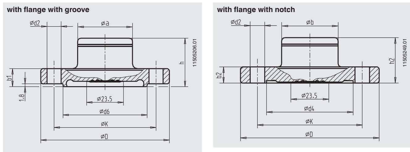
Type of process connection: Aseptic flange connection per DIN 11864-2 form A
