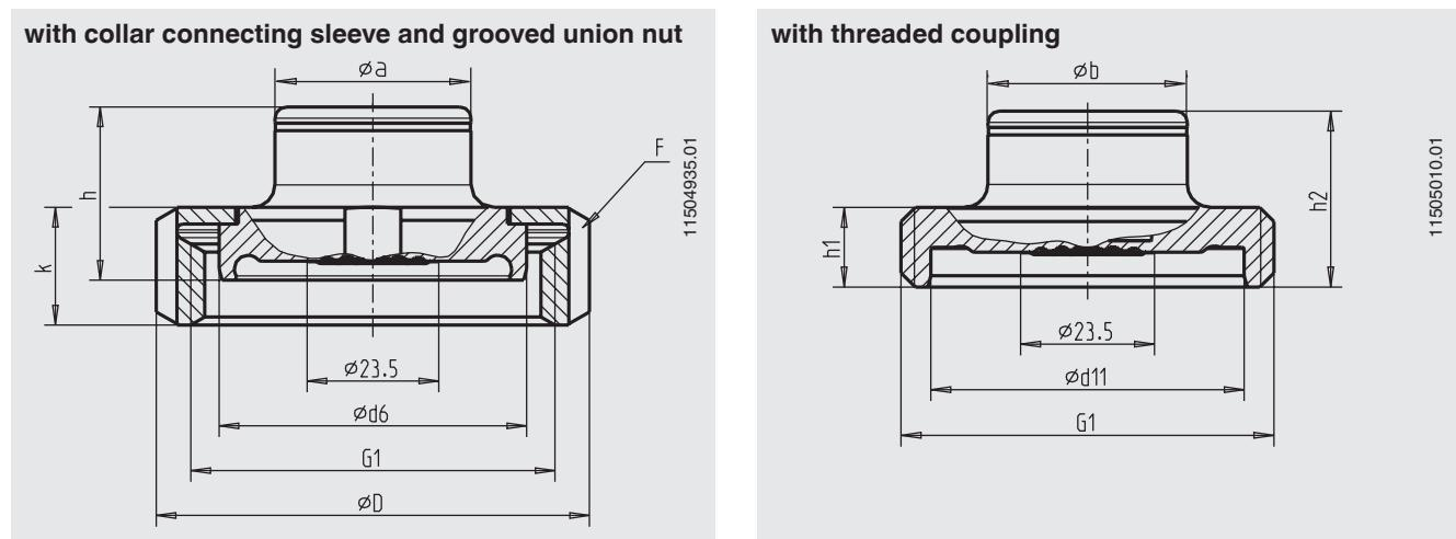
Type of process connection: Aseptic threaded pipe connection per DIN 11864-1 form A
