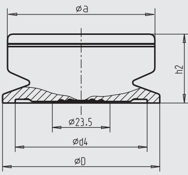
Type of process connection: Aseptic clamp connection per DIN 11864-3 form A
